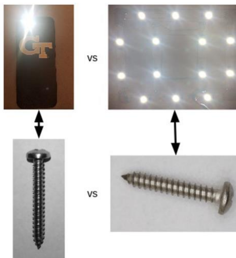
Figure 7. Single LED source and resulting image (left), 12-LED circuit and resulting image (right).
